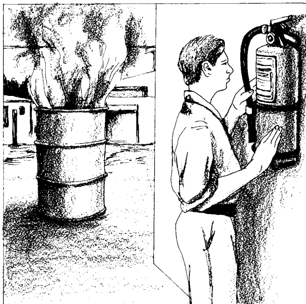
Check extinguisher to see if it is rated to put out the type of fire you are confronting.
